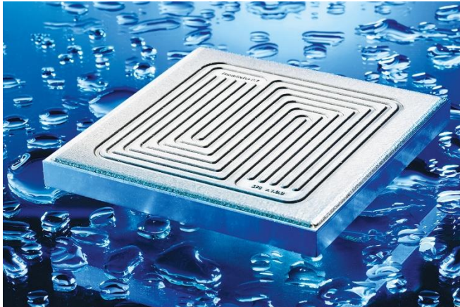
Image 3: The forming tool coated with EHLA saves considerable time and costs compared to conventional tool making. Tobias Keller from the Surface Technology and Ablation Department at Fraunhofer ILT finished it using laser material ablation. © Fraunhofer ILT, Aachen, Germany.
