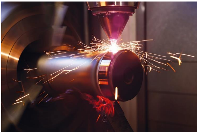
Image 4: SMaC combines the EHLA coating process with a simultaneous subtractive finishing step, thereby significantly increasing productivity. The process heat generated in the coating process makes machining significantly easier. © Fraunhofer ILT, Aachen, Germany.
